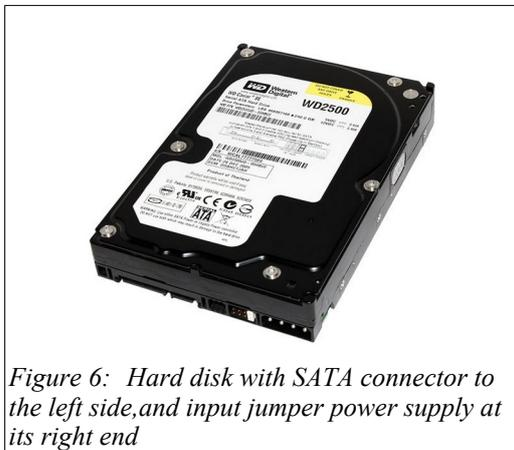
Figure 6: Hard disk with SATA connector to the left side, and input jumper power supply at its right end
