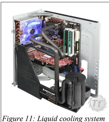
Figure 11: Liquid cooling system
